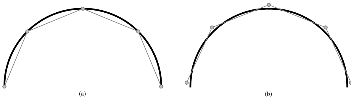
Fig. 3. Mesh of polynomial degree one (gray line) for the circular arc (black line). \mathcal{L}_2 -disparity computed using q = 2 . (a) Initial interpolating mesh ( d = 0.156 ); and (b) optimized approximating mesh ( d = 0.065 ).
