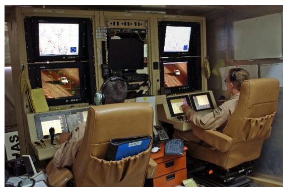
Figure 2.3: MALE Ground Control Station
