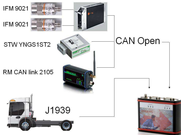
Figure 2. Detail of the data acquisition system wiring.
