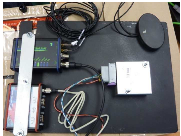
Figure 1. Detail of the data acquisition system: GPS Module (upper left), GPS Antenna (upper right), CAN Case XL (below left), and Inclinometer (center right).
