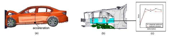
FIGURE 1. (a) Simulation of a vehicle front crash, (b) vehicle front structure and (c) force-deformation characteristics of a structural component of a front car structure.
