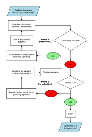
FIGURE 2. The flowchart of the algorithm to identify the maximal hyperbox.
