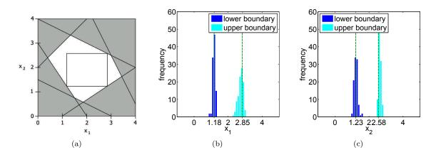
FIGURE 7. Problem 1. (a) Convex polytope in d = 2 dimensions with the hyperbox of maximal volume. (b) Distribution of the hyperboxes found by the algorithm for  $x_1$  in 100 simulations. (c) Distribution of the hyperboxes found by the algorithm for  $x_2$  in 100 simulations.
