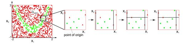
FIGURE 3. Trimming algorithm to select the hyperbox with the most good sample points in  $\Omega$ .
