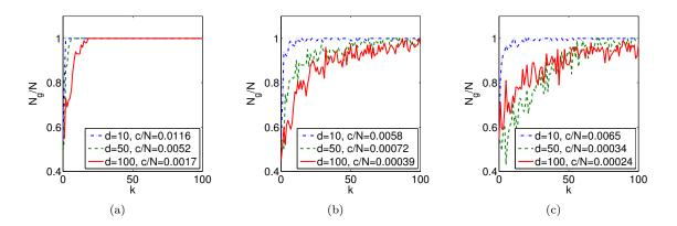
FIGURE 17. Fraction of good sample points versus the number of iterations for N = 100 for (a) Problem 2 (hyperbox), (b) Problem 3 (tilted hyperplane), and (c) Problem 4 (front crash).
