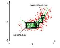
FIGURE 4. Iteration process starting in the classical optimum to move towards a beneficial direction with increasing box size.
