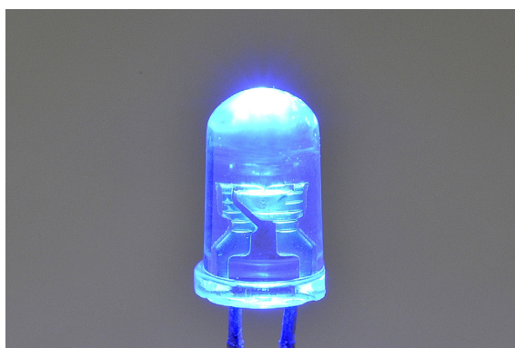
Fig. 1. Photograph of a blue LED in the common 5 mm package. The emitting chip is contained in the well on top of the pin on the right. The dome acts as a lens to disperse the light.
