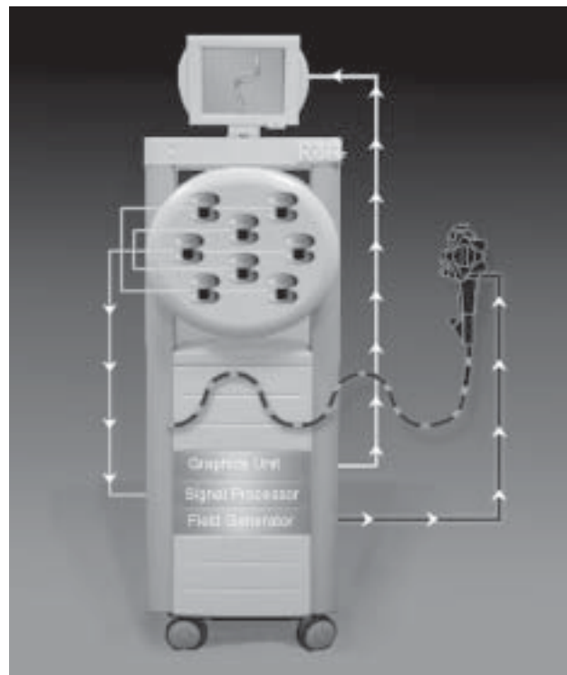
Figure 2. ScopeGuide imager. Specially designed colonoscopes have inbuilt coils which are energised and generate magnetic fields of different frequency. The magnetic fields are detected by the round sensor disk, which is placed in front of the patient. Information from the disc is analysed to produce a 3D image of the endoscope shown here in the top screen. Trainees can modify their technique according to the image on the screen.
