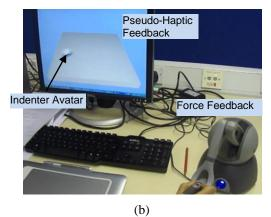
**Fig. 4** (a) Modification of the cursor speed when passing over a hard nodule; (b) combined force feedback and pseudo-haptic feedback.
