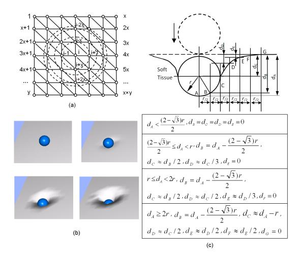
Fig. 3 (a) Mesh representation for the soft object deformation visualization: the number of the vertices of triangles of soft object surface is  $x \times y$ , where the node *i* is positioned at the center of the indentation area; (b) tissue deformation increases as indentation depth increases; (c) simplified model of deformation curvature of soft tissue surface
