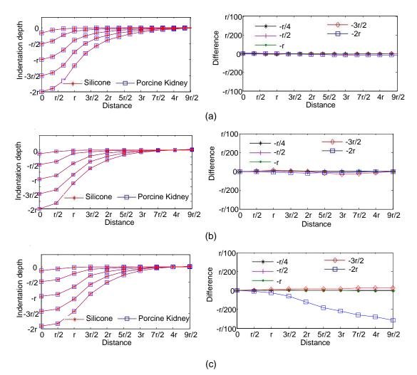
**Fig. 2** On the left panels the deformation curvature of silicone (RTV6166 gel) and porcine kidney at different indentation depths are reported, by using 6mm (a), 8mm (b), and 10mm (c) indenter, according to 3D finite element simulation; on the right panels the difference between the displacement curvatures are reported
