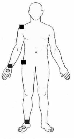
Source electrodesDetector electrodes
