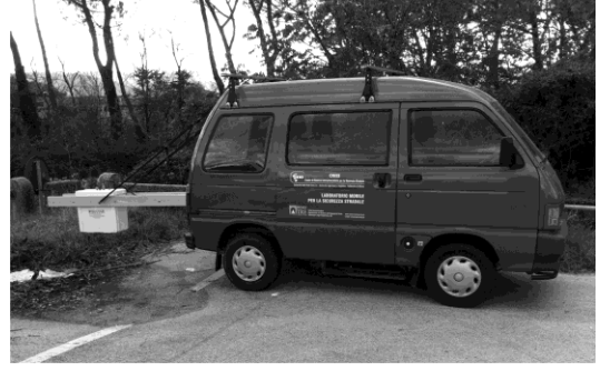
Fig. 2. GPR survey van mounting the air-launched antenna RIS Hi-Pave HR1 1000, manufactured by IDS Ingegneria dei Sistemi S.p.A., Italy
