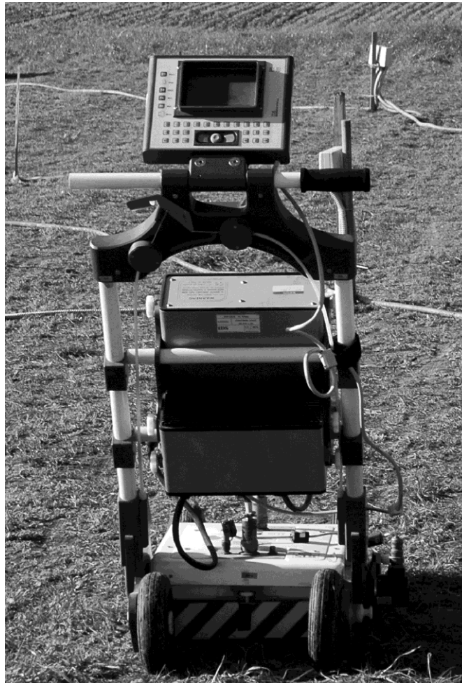
FIGURE 1 a) Ground-coupled antenna pulse radar system, 600 MHz and 1600 MHz center frequencies of investigation, manufactured by IDS S.p.A.
