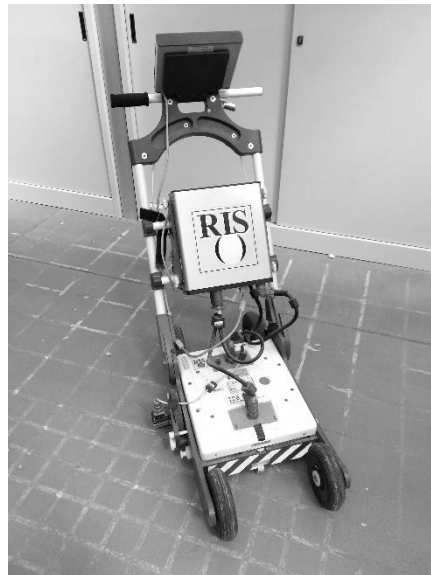
Figure A.2: RIS 2k-MF Multi Frequency Array Radar-System, manufactured by IDS Ingegneria dei Sistemi S.p.A., Italy.
