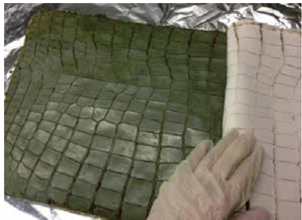
Figure 12. A wax 'skin' being taken from the mould
