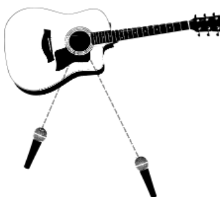
Figure 2 A single source being reproduced by 2 microphones with the path of the direct sound indicated by dashed lines.
