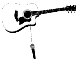
Figure 1 A single source being reproduced by a single microphone with the path of the direct sound indicated by a dashed line.
