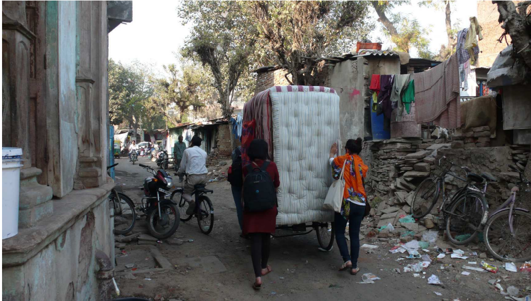
Fig. 2: The test-version of the mNAP in Ahmedabad. Here, a lightweight sound-insulated box was constructed on the back of a bicycle rickshaw, providing some sonic separation from the urban environment. This box was tested both within the National Institute of Design and the urban village of Kocharab.
