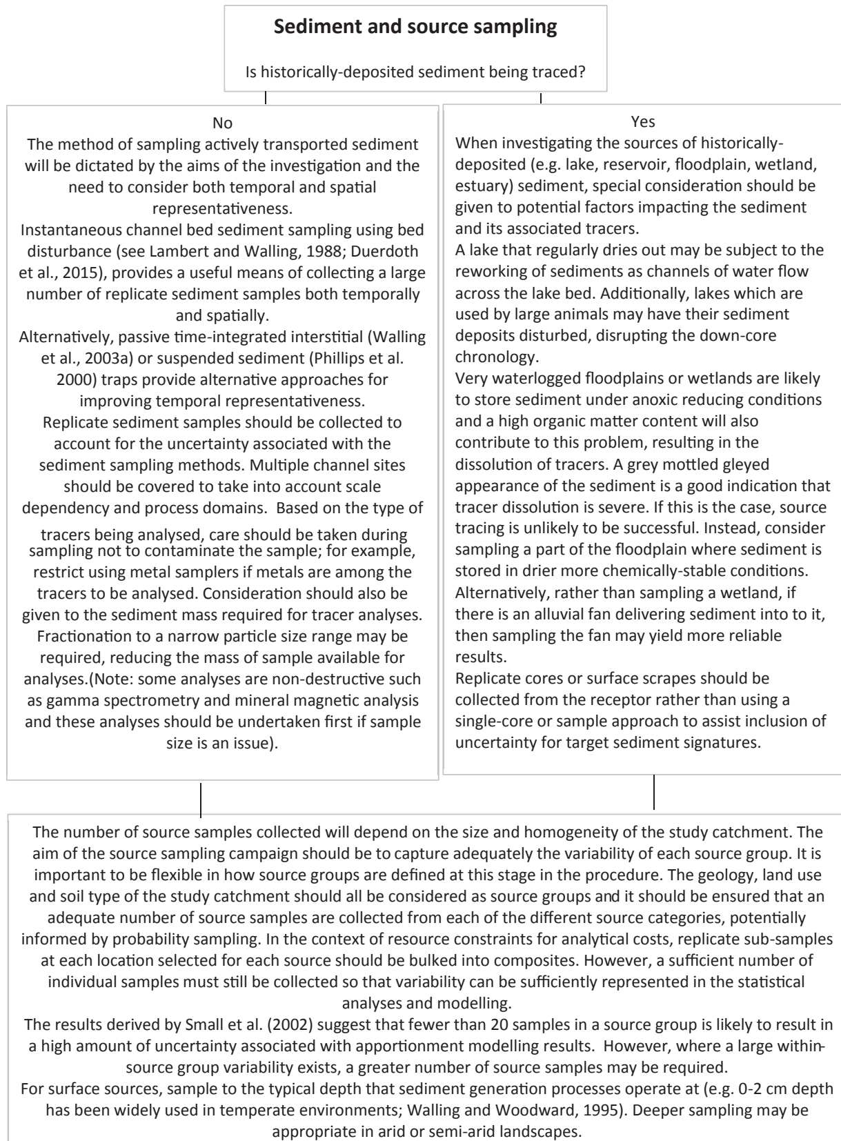
Fig. 1. A methodological decision-tree for guiding application of sediment source fingerprinting (Rousseeuw and Croux, 1993).
