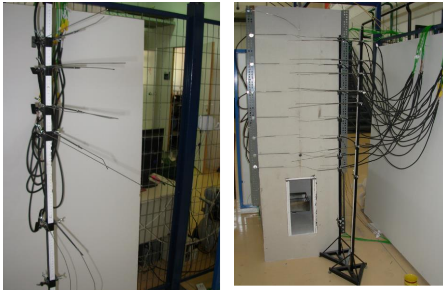
Figure 4-4. Positioning of the thermocouples at the exterior of the fire compartment.
