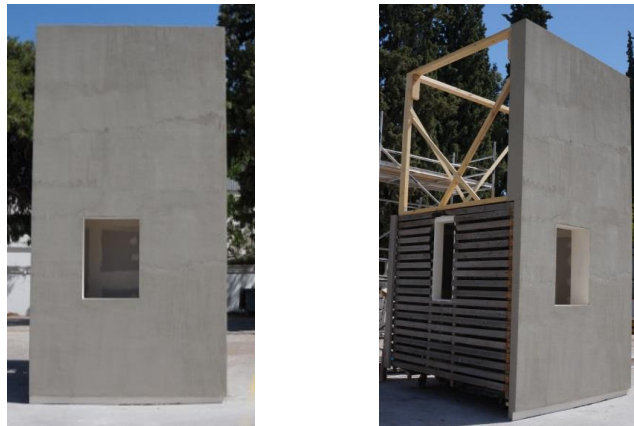
Figure 6-2. Photographs of the large scale compartment façade configuration: front and side view.
