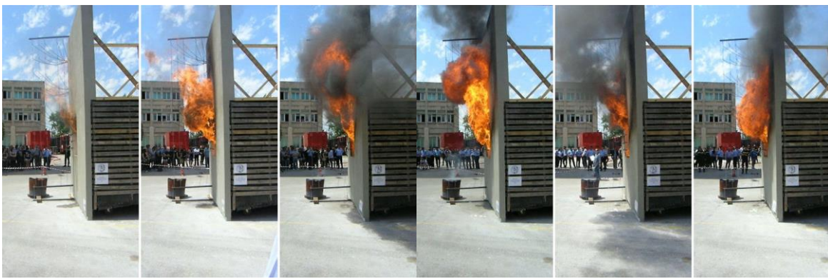
Figure 6-17. EVF development at 2.5 min intervals (side view).
