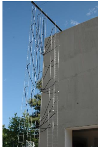
Figure 6-10. Construction details of the thermocouple positioning at the exterior of the fire compartment.
