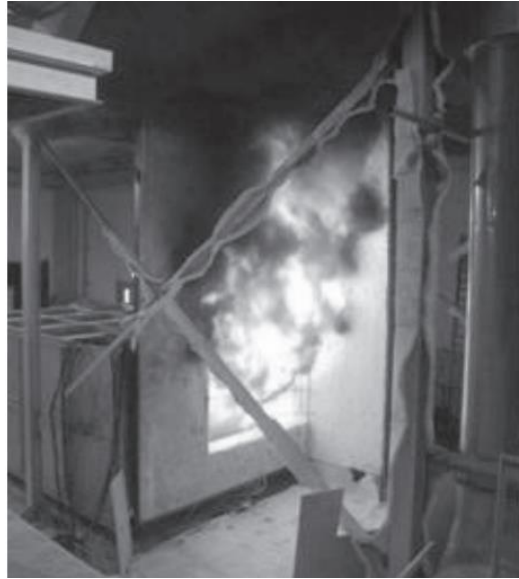
Figure 2-4. Flame emerging out of the opening during the experiment in the ISO13785-2 configuration (Yoshioka et al., 2012).
