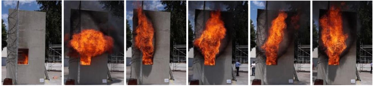
Figure 6-16. EVF development at 2.5 min intervals (front view).
