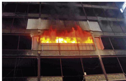
Figure 1-3. BRE Cardington full-scale fire test (Welch et al., 2007).
