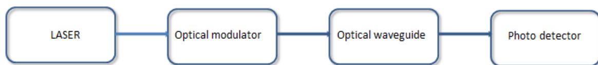
Figure 3. Optical system consisting of transmitter, optical modulator, optical waveguide and photo detector
