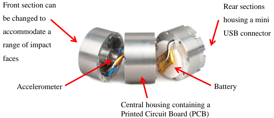
Figure 6.2: Med-Eng Ballistic Data Acquisition System (BDAS) unit mounted within a four piece aluminium shell.
