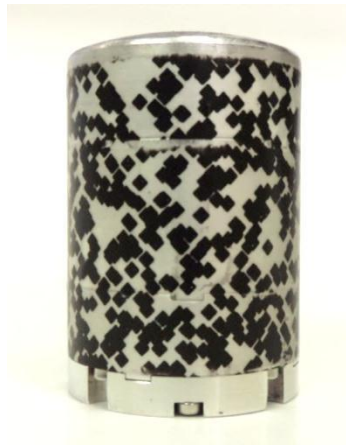
Figure 6.4: Projectile with high contrast pattern applied to the outer surface of the shell.
