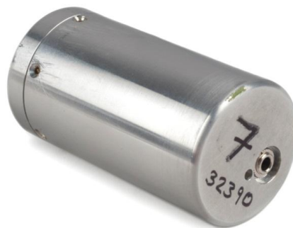
Figure 9: Rear view of the prototype Acceleration Logger. The connector and LED viewing hole are visible on the rear in conjunction with the projectile serial number.
