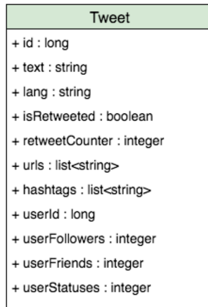
Figure 5.1: Tweet object structure in the S4 application
