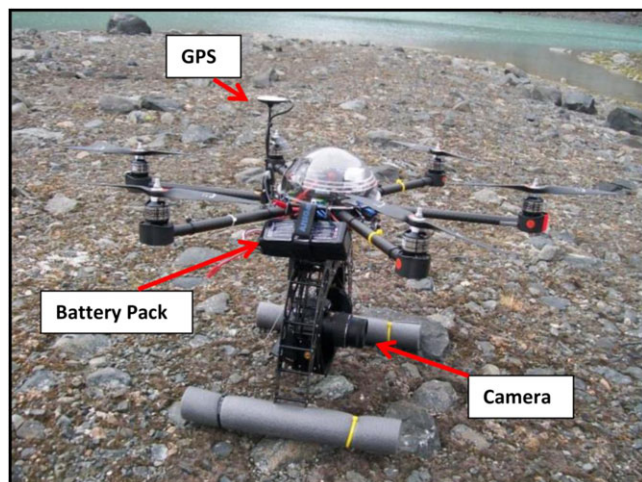
Figure 2. The hexacopter with key components labelled. This figure is available in colour online at wileyonlinelibrary.com/journal/esp
