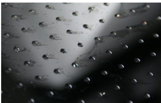
Figure 1. The etched holes on the rear (polished) surface of a silicon wafer.
