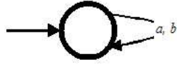
Figure 1. A single-state X -machine that recognises the non-regular language \{a^n b^n \mid n \in \mathbb{N}\} . In this example, we take X = \{A, B, Fail\} \times \mathbb{N} . The encoder and decoder are defined by e(s) \equiv (A, 0) and d(s, n) \equiv (s \neq Fail \wedge n = 0) . The labelling is given by
