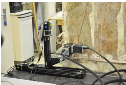
Fig. 2. Terahertz imaging set-up, taken before conservation was completed. © LRMH
