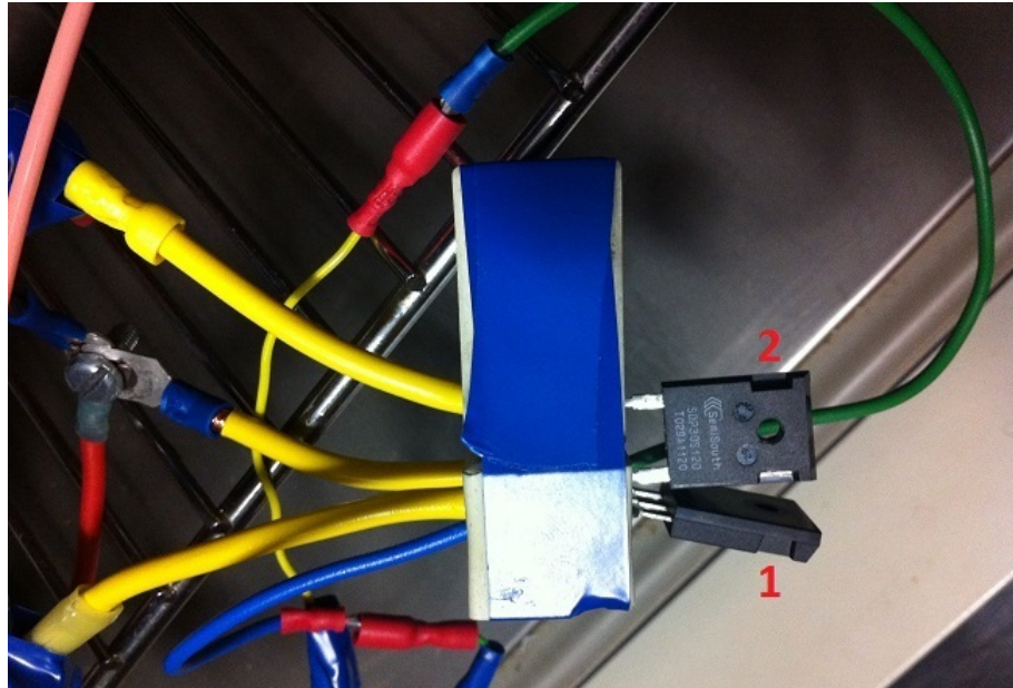
Figure 3.4: Devices connection for LV measurements: 1- Transistor 2- Diode.
