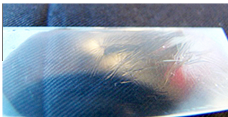
Fig. 7. PPX deposited on water on a glass substrate at a pressure of 80 kPa; a black tissue was put underneath for better contrast. The water is spread over the entire substrate of a 76 \times 26 mm glass substrate. Possibly a small water loss occurred during deposition; this could explain the appearance of small wrinkles.
