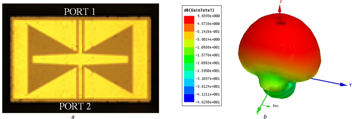
Fig. 11 Two port bow-tie slot antenna with two CPW feed lines (a) Fabricated bow-tie slot antenna with two CPW feed lines where port 1 and port 2 are used to characterise the antenna, (b) Simulated radiation pattern at 280 GHz. The antenna has a maximum gain of 9.7 dB
