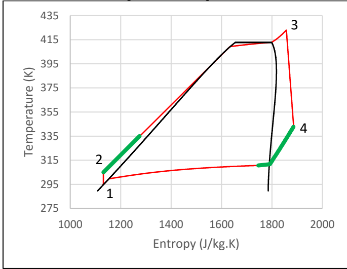
Figure 3: Temperature – Entropy diagram of a conventional zeotropic ORC cycle, with the regenerative portion marked in green
