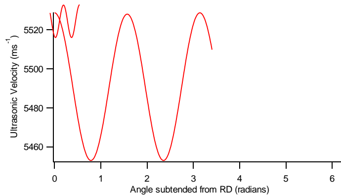
Figure B.13: S 0 mode Lamb wave velocity angular variation prediction from all twelve EBSD Eulerian angle datasets obtained from the 1mm thick aluminium sheet AL104325.
