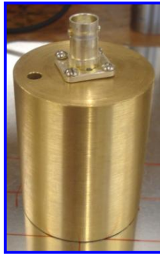
Figure 3.1: Photograph of a typical EMAT used for this study. The brass casing houses the permanent magnet and coil. The brass casing is 50 mm tall with a diameter of 45 mm.
