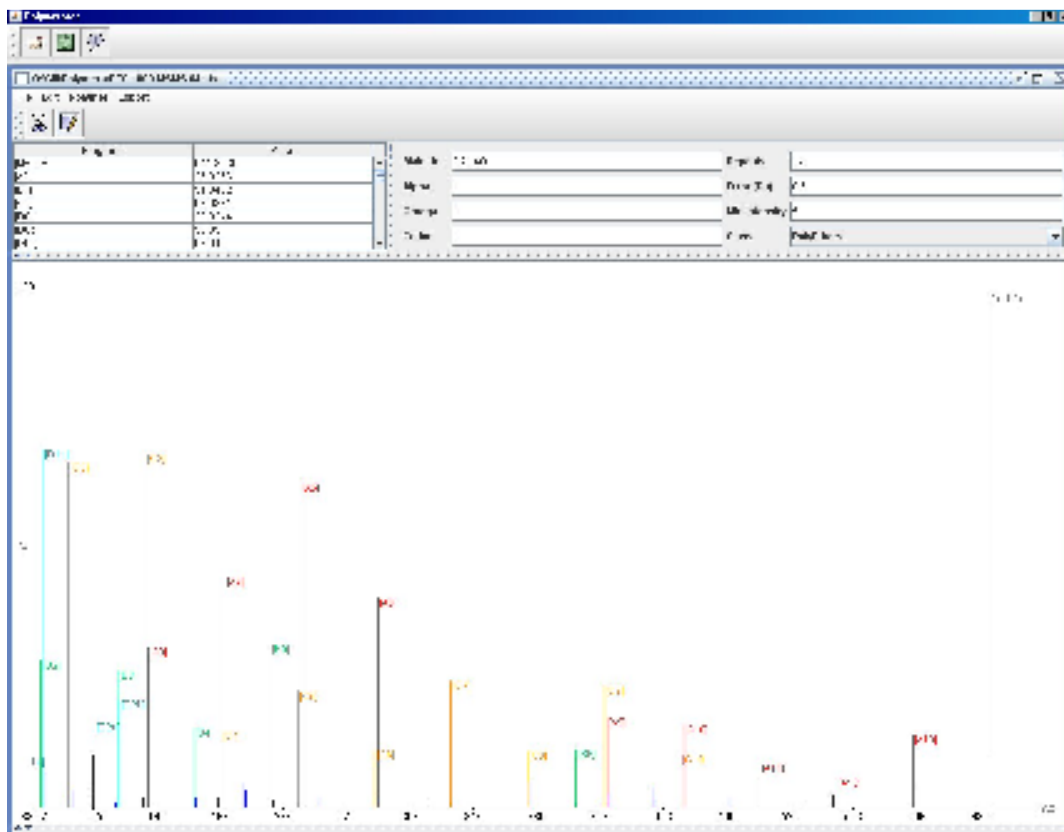
Figure 6.7: Screenshot from the Polymerator software of an annotated ESI-MS/MS spectrum from the lithiated 14mer of dihydroxyl end capped poly(ethylene glycol). Predicted fragment ions are detailed above (left) the spectrum.
