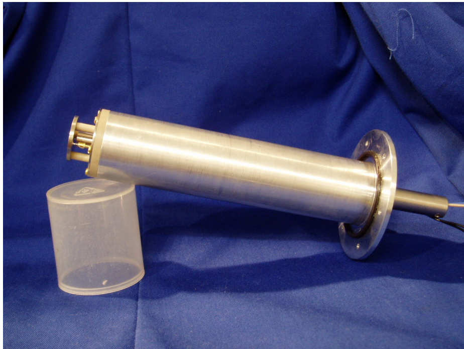
Figure 5.3. Photograph of the carbon nanotube emitter assembly and the supporting cylinder.
