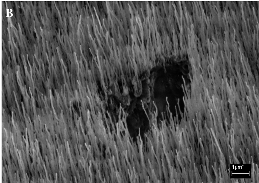
Figure 3.7. SEM micrographs showing (A) a large area of a typical dense array (B) a close-up of one of the holes and surrounding nanotubes.
