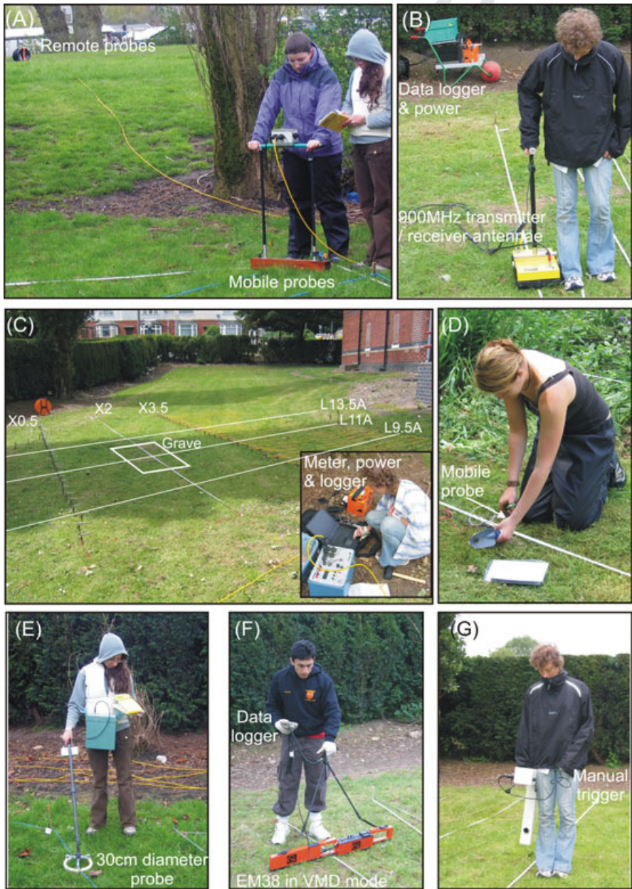
FIG. 3—Photographs of some near-surface geophysical equipment being trialled. (A) Bulk ground resistivity equipment; a Geoscan RM4 lateral array. (B) High-frequency (900 MHz dominant frequency) GPR PulseEKKO™ 1000 equipment. (C) ERT electrode arrays (x 0.5 and x 3.5 arrays laid out) using (inset) the CAMPUS TIGRE system. (D) SP survey using Pb-Cl probes and a standard voltmeter. (E) A Bartington MS1 magnetic susceptibility meter. (F) Bulk ground conductivity equipment: a Geonics EM38B. (G) Magnetism equipment: a Geoscan FM18 fluxgate gradiometer.
