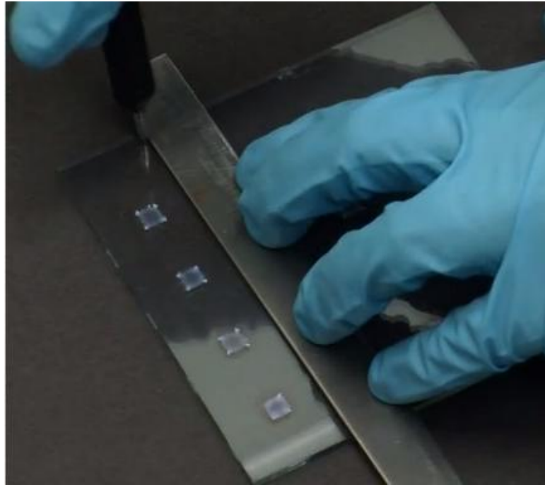
Figure 4.39 – Cutting the FTO glass with a diamond glass cutter
