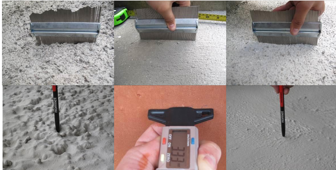
Figure 3 Left to Right: as-sprayed, smoothed and regulated surface finishes, Top to Bottom: before and after application of TamSeal 800 spray applied waterproofing membrane
