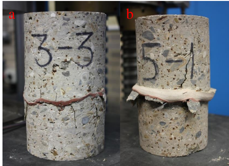
Figure 10 Typical compressive failure modes for (a) thin membrane interface (b) thick membrane interface
