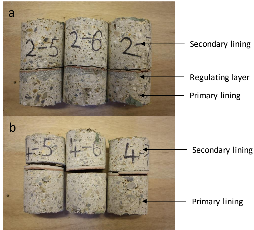
Figure 13 (a) membrane bonding to regulating layer and debonded from secondary lining (b) equal probability of debonding from primary or secondary linings if no regulating layer present
