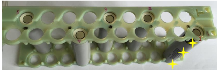
Figure 2: Experimental set-up showing temperature monitored cells within a 19 cell module
