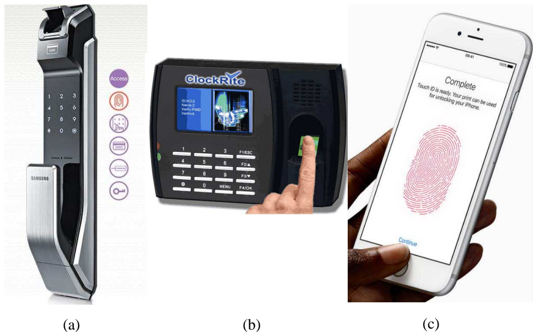
Figure 1.4: Some examples of personal and commercial applications of fingerprints biometrics: (a) Samsung fingerprint door lock (Taken from [25]); (b) Fingerprint clocking system utilize fingerprint biometrics to assure the user is really he claims to be when clocking in and out (Taken from [26]); (c) iPhone 6s embedded with fingering sensor which assist establishing a digital ID for unlocking mobile phone and also for authorizing online payments (Taken from [27]).
