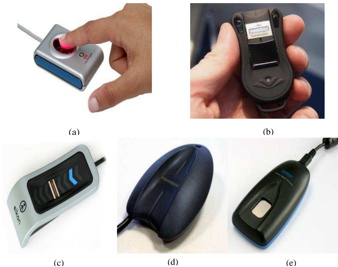
Figure 1.7: Some examples of fingerprint sensors: (a): optical sensor (Taken from [34]); (b): ultrasound sensor (Taken from [35]); (c) capacitive sensor (Taken from [36]); (d) thermal sensor (Taken from [37]); (e) pressure sensor (Taken from [38]).
