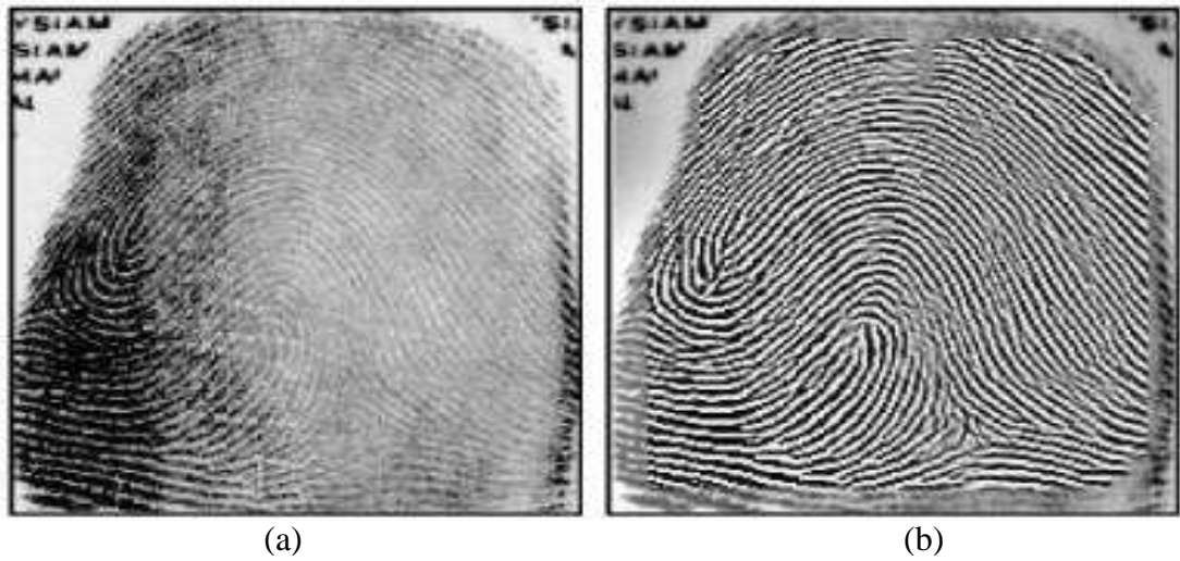
Figure 3.2: (a) The original image (b) the enhanced image using Gabor filters approach as suggested by Hong (Taken from [4][64]).
