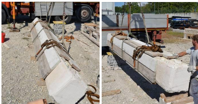
Figure 13. Rotation of a beam which were tested in horizontal plane.
