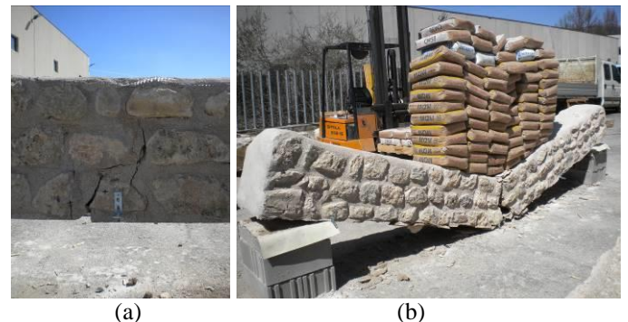
Figure 14. (a) Crack pattern produced by gravity self-weight load. (b) Ring-beam No. P3-U-V after testing.
