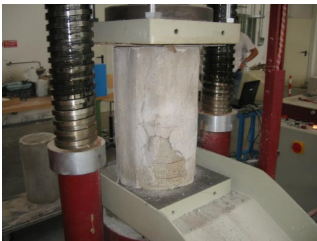
Figure 8: Compression test (reinforced column).
