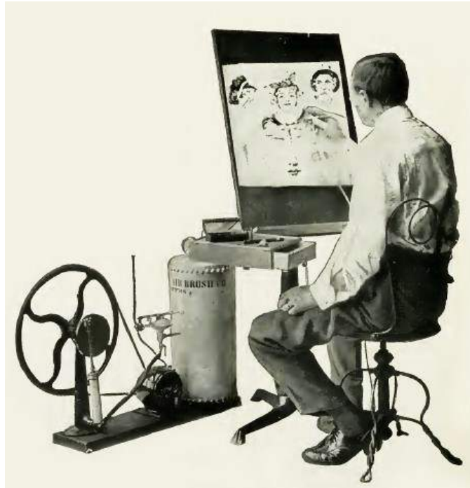
Figure 3: a photograph from the early 20 th Century of an illustrator while using an airbrush powered by an early type of electrical air compressor (Stine, 1920, p. 148)
