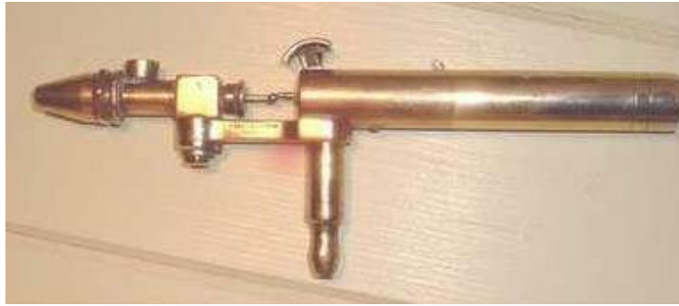
Figure 11: an early Aerograph model by Charles Burdick (courtesy of Andy Penaluna)
