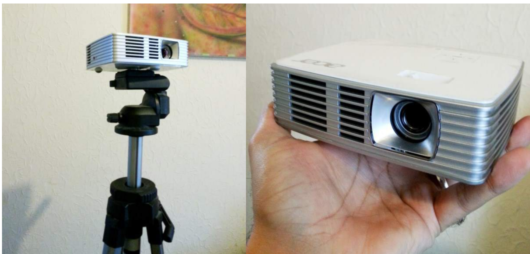
Figure 94: the Acer K130 projector used for the virtual image-reintegration experimental carried out for the mock-up painting. For that purpose, the projector was mounted on a tripod to facilitate the necessary adjustments of the image projected.
