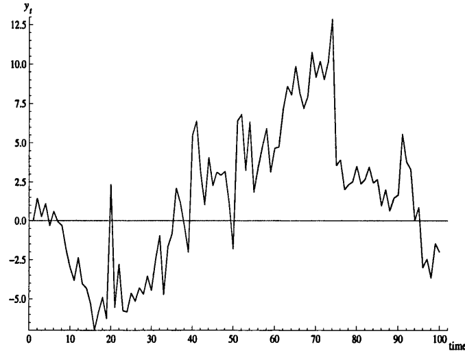
Figure 3.4: Artificial data set generated from a local level model, with T=100 , with outliers at time t = 20 and t = 50 , of size 7 and -6, and level shifts at time t = 40 and t = 75 of size 7 and -7.
