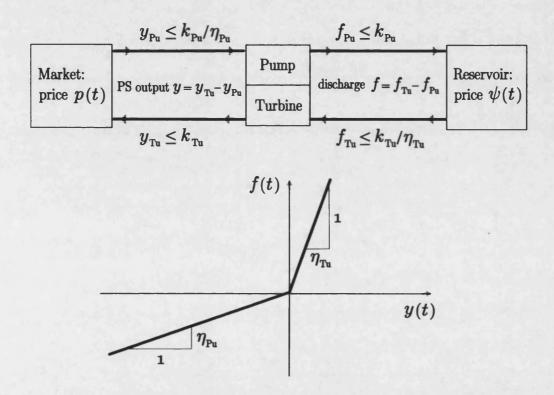
FIGURE 3.1. Conversion efficiencies  $(\eta_{Pu}, \eta_{Tu})$  and the relationship between the storage plant's output rate y(t) and the outflow from the reservoir f(t).
