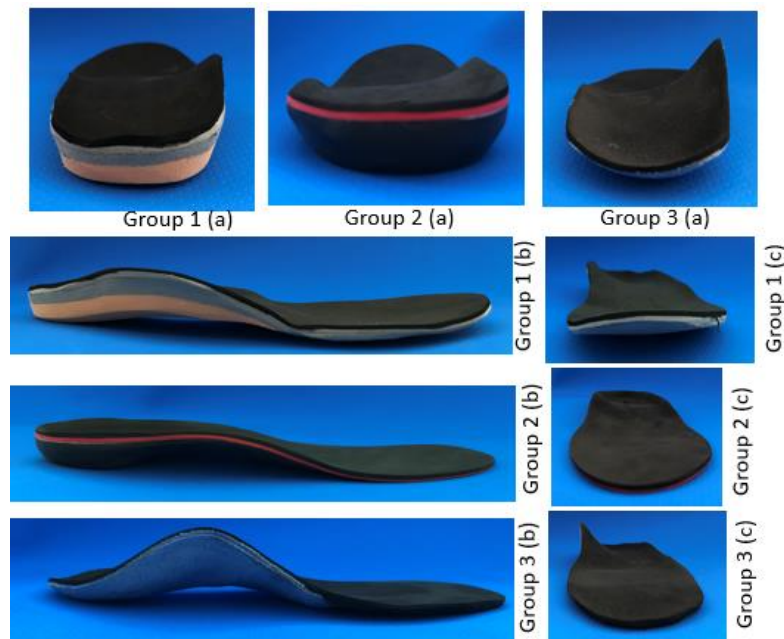
Figure 10. Foot orthoses included in the study. Group 1 (A) direct adaptation technique posterior view, group 1 (B) direct adaptation technique medial view, group 1 (C) direct adaptation technique anterior view. Group 2 (A) CAD/CAM foot orthoses posterior view, group 2 (B) CAD/CAM medial view, group 2 (C) CAD/CAM anterior view. Group 3 (A) prefabricated orthoses posterior view, group 3 (B) prefabricated orthoses medial view, group 3 (C) prefabricated orthoses anterior view. CAD, Computer-Aided Design; CAM, Computer-Aided Manufacturing.
