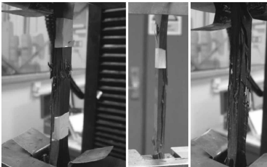
Fig. 3 Dominant failure modes for the tensile testing of laminates. LHS/RHS: explosive gage middle; centre: long splitting gage middle
