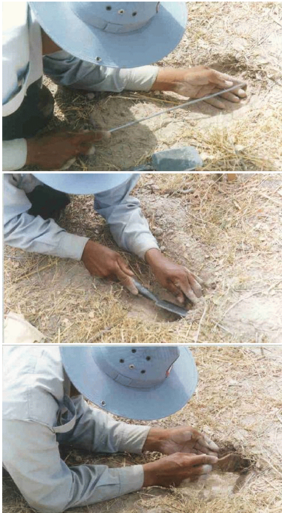
Figure 2.9: Prodding and excavation in hard dry soil in Cambodia. Gradual uncovering towards a target by prodding to a limited depth, then removing soil with a trowel and a paintbrush.
