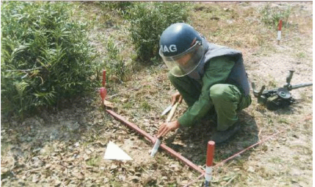
Figure 2.12: Deminer being trained to new SOPs which permit working in a squatting position. Note the one-metre wide lane, stick to indicate baseline, and that the deminer has both hands behind baseline while prodding/excavating.
