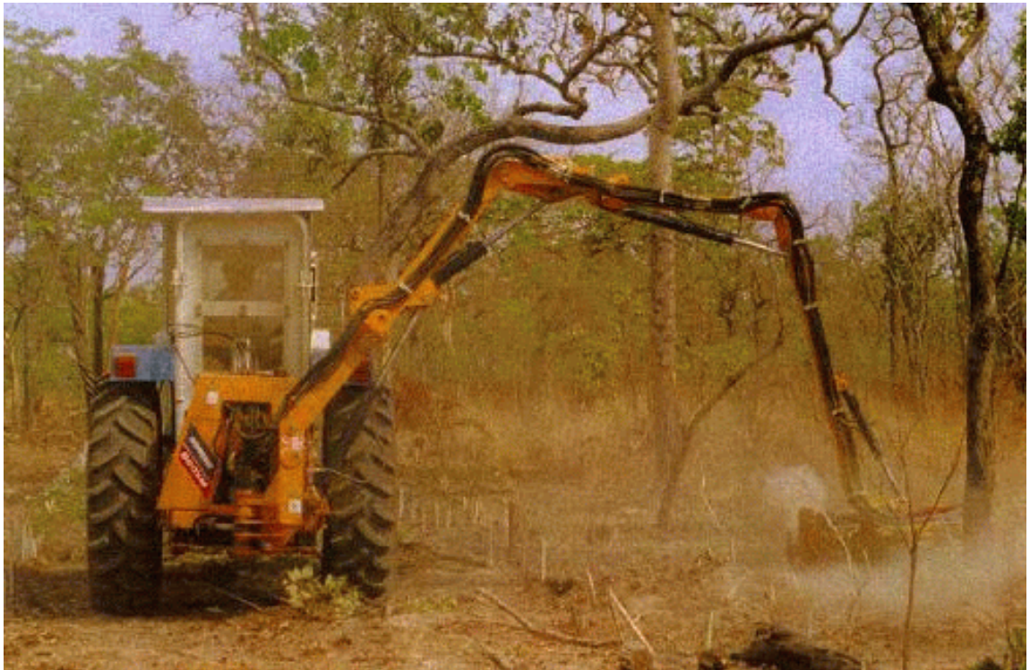
Figure 2.3: Vegetation clearance using a flail on a long boom on an armoured tractor. Note: tractor and cab are heavily armoured on right-hand side only. From CD-ROM catalogue of demining equipment [M + 99].
