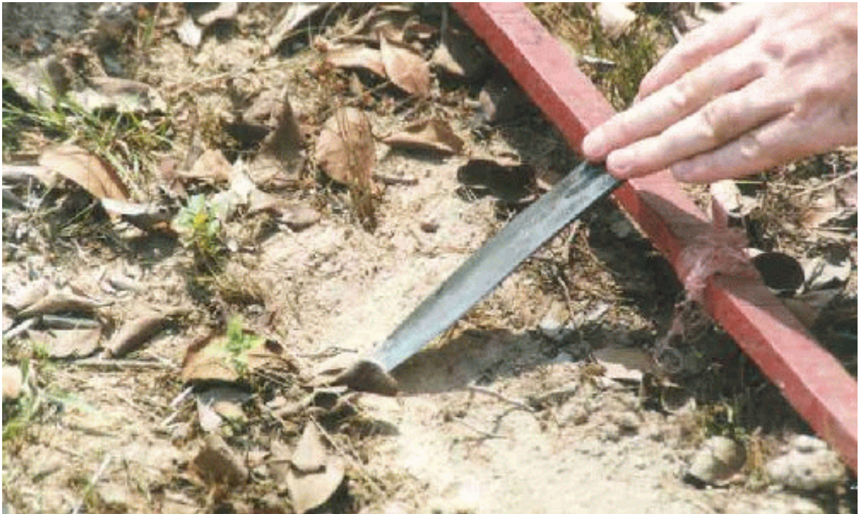
Figure 5.1: Combined prodding/excavating tool. This tool is locally made in Cambodia at low cost.
