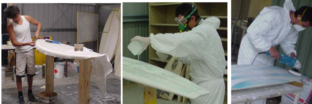
Cutting the fibreglass cloth
