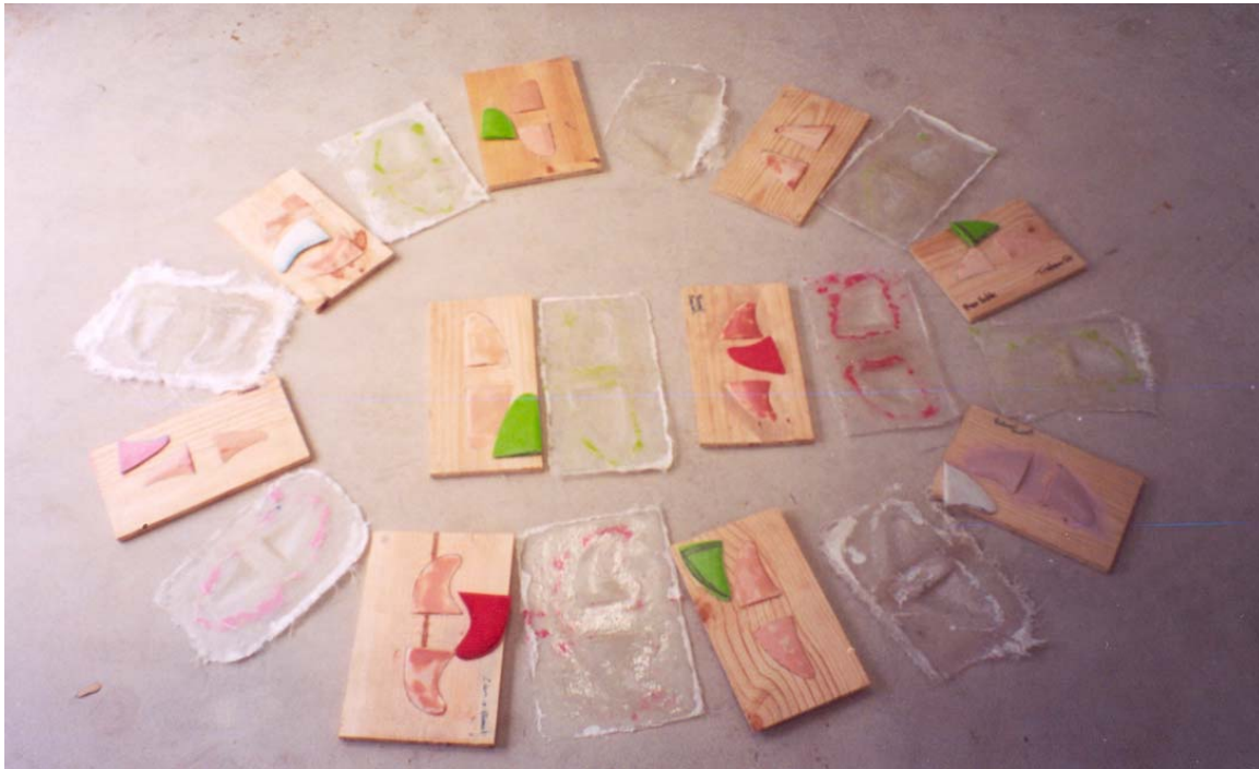
Figure 6 An example of different fins designed according to various NACA standards [10] and produced by laminating technique at Edith Cowan University in the 1 st semester of 2004.
