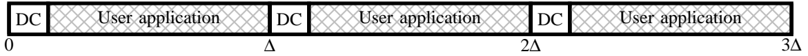
Fig. 3. Division of time between the duty-cycling mechanism and user applications. The protocol works in a sequence of time periods of length \Delta . In each period, the first phase is dedicated to duty-cycling (DC), and the second phase to the user application.
