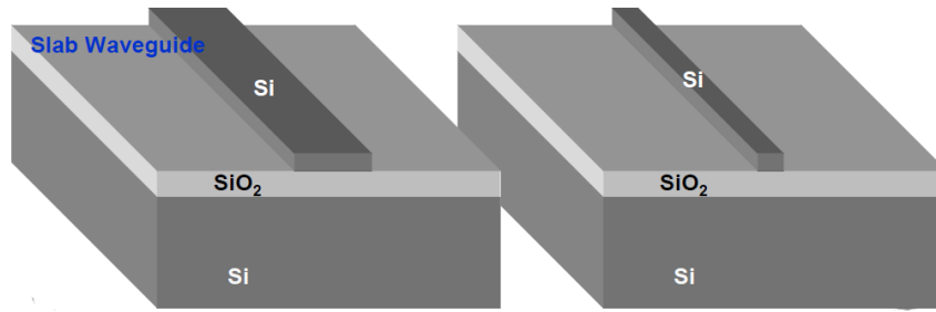
FIGURE 3.5: We can approximate the modes in x direction as a slab waveguide for the left structure. However we can not compute the y direction modes using the slab waveguide approximation. The right structure is the one we will be dealing with for our designs. It can have air cladding or SiO_2 cladding.
