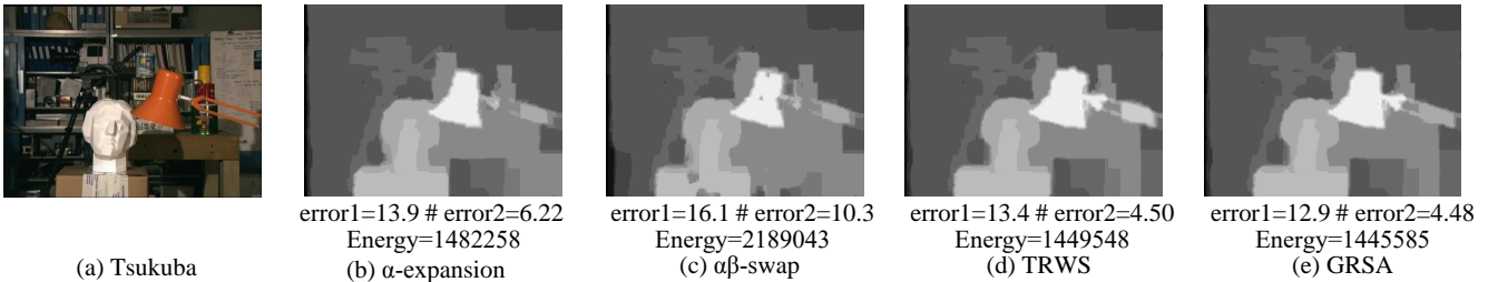
Fig. 10 The stereo matching results obtained by \alpha -expansion, \alpha\beta -swap, TRW-S and the GRSA with the truncated convex function. The errors (%) are tested on Middlebury Stereo Evaluation. Error1 is tested with the error threshold ET = 1 , and error2 is tested with ET = 2 .
