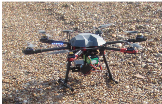
Fig. 2. The Hexacopter platform deployed in the field trial.
