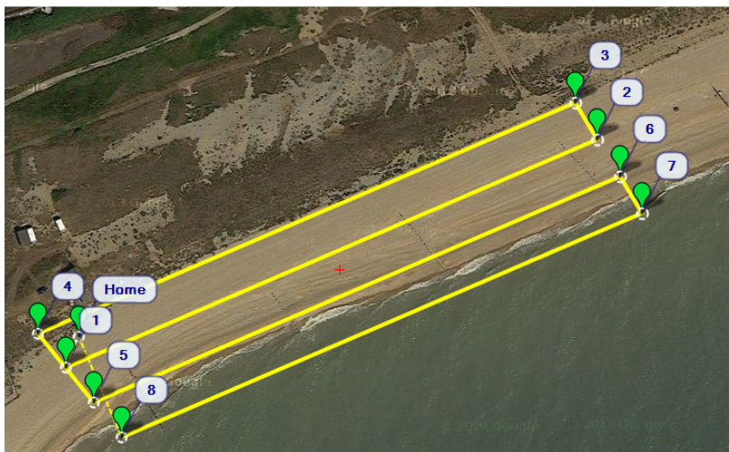
Fig. 3. Flight plan for experimental survey at Normans Bay section of Pevensey Bay.
