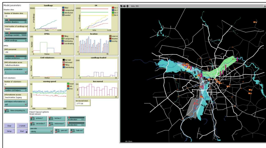
Figure 3.2.3. Screenshot of the NetLogo model interface. The map shows a snapshot of a running simulation, with DMOs moving along the street network and disaster sites in various states of protection. The green shaded area depicts a river section that is already protected whereas in the grey shaded areas sandbags are still needed at various sites.
