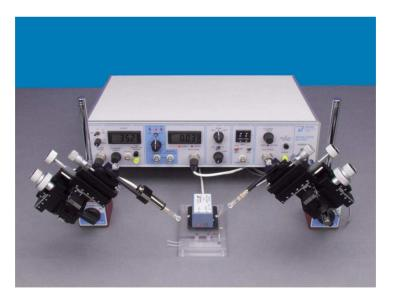
Figure 2: Voltage Clamp Apparatus Two Electrode Voltage Clamp Apparatus. From https://www.warneronline.com/product\_info.cfm?name=TEV-700+Two+Electrode +Voltage+Clamp+Workstation&id=170.
